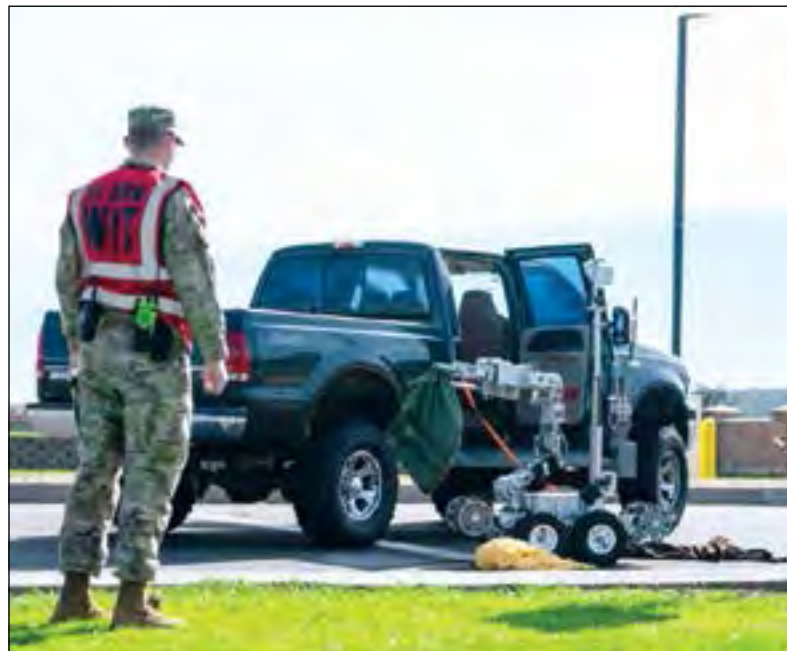
A U.S. Airman, assigned to the 60th Civil Engineer Squadron, observes an explosive ordnance disposal robot during the exercise, Roundel Galaxia, Feb. 25 at Travis Air Force Base, California. The robot is designed to assist the EOD team's ability to examine explosive and dangerous substances without being in range of harm's way.
